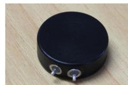
Physically the device is a metal cylinder, 24mm in diameter and about 8mm thick. The case is manufactured from either anodised aluminium or stainless steel, depending on the depth rating required. It is available with an optional dome on the front face which provides a single point contact with the head resulting in improved frequency response.
